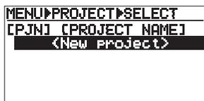
While the above screen is shown, pressing the [ENTER] key creates a new project (you can make recording to the project in the insert mode).
