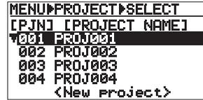
By selecting "<New project>" shown at the bottom of the list, you can create a new project on the hard disk (see "Creating a new project" below).
