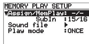
In this screen, you can make setting for memory play including the channel assignment, playlist setting and play mode setting, as well as destination assignment of the "Sub In" signal.
